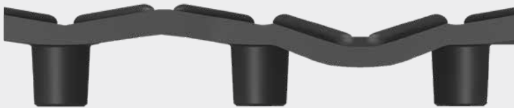
Cross section of ergonomic domes compressing
